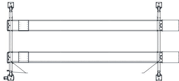
Fig 11 – Lock Release Air Line Routing
