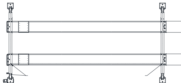
Fig 11 – Lock Release Air Line Routing
